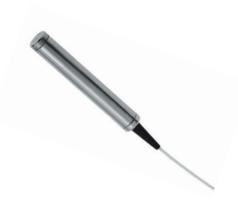
Agiltron Fiber Optic Retroreflector is designed to reflect light input backward through the fiber. Our retroreflectors are available with single mode (SM), polarization-maintaining (PM), or multimode (MM) fiber. A specially made mirror is used in our device that achieves high reflection up to 99% and high optical power handling up 5W.
